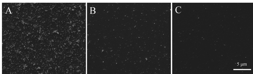
Figure 4. SEM images of the (PVPON/TA) 60 films fabricated at 10 (A), 22 (B), and 25 °C (C), respectively.
